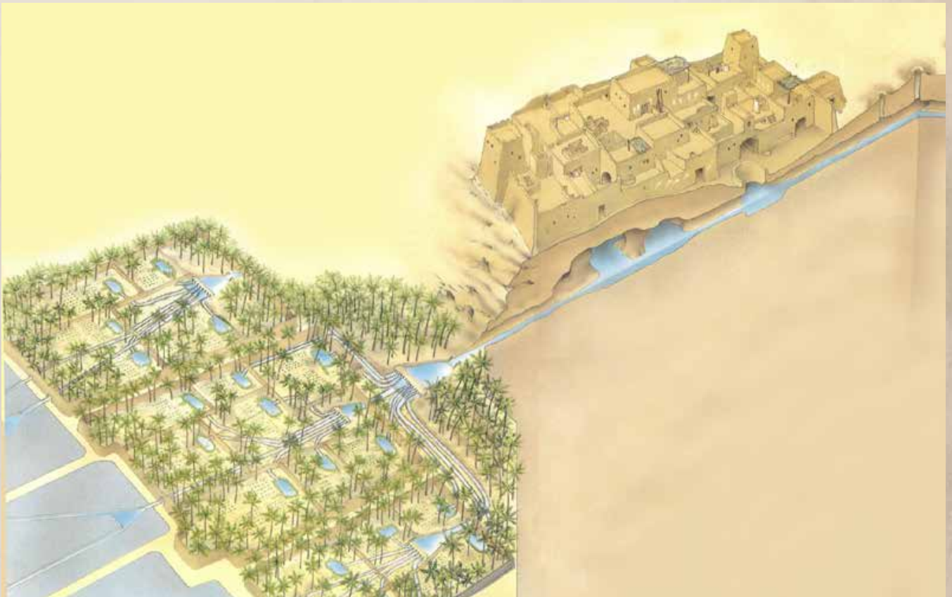
Rendering of the organization of gardens and water distribution in an oasis (plan, surface channels, water sharing).
